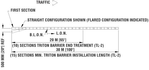
Figure 10 Triton Barrier<sup>®</sup> (TL-2) 70 km/h [45 mph] End Treatment Placement
