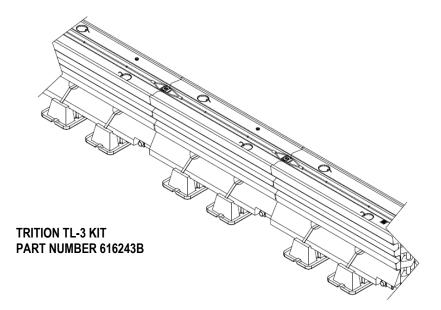
Figure 4 TRITON BARRIER<sup>®</sup> TL-3 assembly (100 km/h [62 mph])
