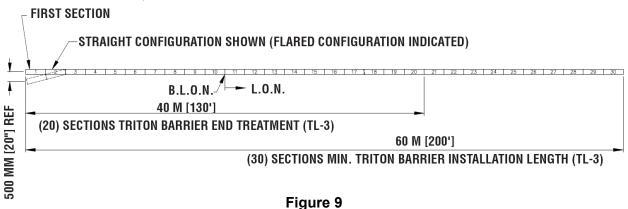
Figure 9 Triton Barrier<sup>®</sup> TL-3 100 km/h [62 mph] End Treatment
