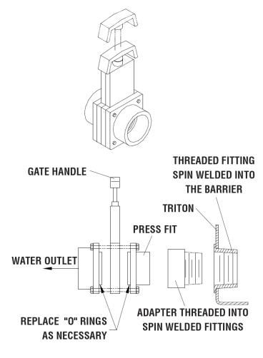
Figure 13 Repair of the Gate Valve
