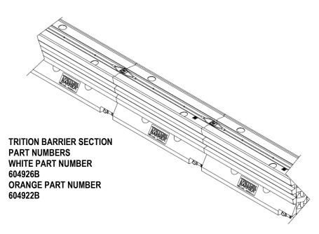
Figure 3 TRITON BARRIER<sup>®</sup> TL-2 assembly (70 km/h [45 mph]
