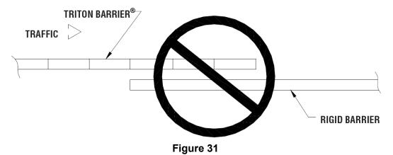
Do **NOT** use Triton Barrier<sup>®</sup> (TL-2 or TL-3) alongside approach end of rigid barrier unless rigid barrier is flared as shown in Figure 30.
