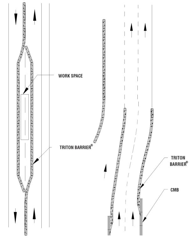
Figure 11 Work in Center of Low-Volume Road (Similar to TA-15 of MUTCD Part 6)
