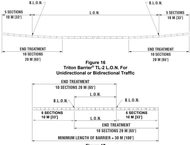
Figure 17 Minimum Length Layout for Triton Barrier<sup>®</sup> TL-2
