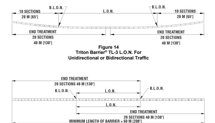
Figure 15 Minimum Length Layout for Triton Barrier<sup>®</sup> TL-3
