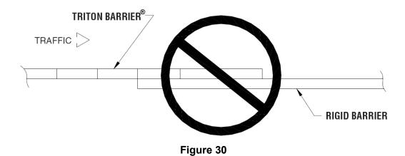
Do **NOT** use Triton Barrier<sup>®</sup> (TL-2 or TL-3) against approach end of rigid barrier (Figure 33) unless rigid barrier is flared as show in Figure 27.
