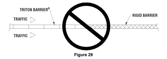
Triton Barrier<sup>®</sup> (TL-2 or TL-3) is **NOT** an End Treatment for rigid barrier. It is only to be used as a terminal to terminate Triton Barrier<sup>®</sup>.
