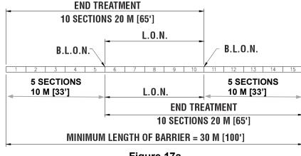
Figure 17a Triton Barrier<sup>®</sup> TL-1 L.O.N. For Unidirectional or Bidirectional Traffic
