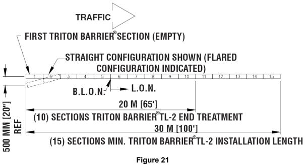
Triton Barrier® TL-2 End Treatment Placement 70 km/h [45 mph]
