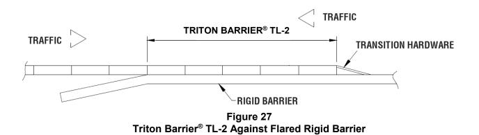
For traffic direction shown here, flare rigid barrier to prevent pocketing. If used in two way traffic where cross-over traffic is a concern, transition hardware is recommended. Five sections must be overlapped.
