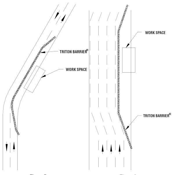
Figure 7 Lane Closure for One Lane-Two Way Traffic Control (Similar to Figure 6C-3 And TA-10 of MUTCD Part 6)
