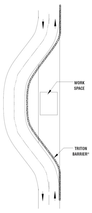
Figure 13 Typical Transition and End Treatment
