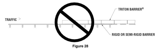
Do **NOT** place end of Triton Barrier<sup>®</sup> (TL-2 or TL-3) directly against rigid or semi-rigid barrier.
