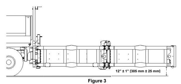
2. Jacks shall be used to support the SS180<sup>®</sup> M when it is detached from the truck. The Jacks must be stored while the TMA is attached to the truck.
