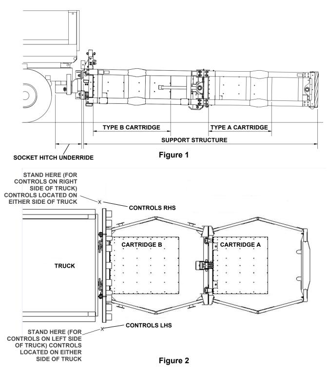
1. The SS180<sup>®</sup> M shall be rigidly fastened to the truck. In the horizontal position, the bottom of the TMA shall be 11" to 13" [280 to 330 mm] from the ground to the bottom of the Rear Impact Face (Figure 3).
